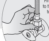
Firmly hand tighten the hose to the valve and add a quarter-turn using the proper wrench. Tighten more if needed.
